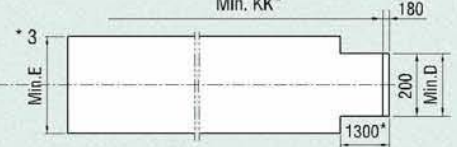
Apertura superiore/Upper floor opening
