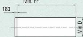
Fossa inferiore/Lower floor opening
